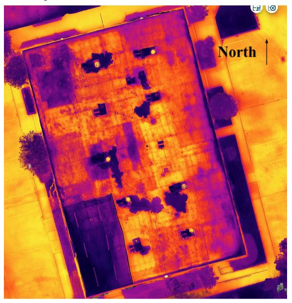
Above is a 2D thermal map of the roof. This map is comprised of 241 individual photos that have been stitched together to create a complete map of the roof overlaid with thermal information.
